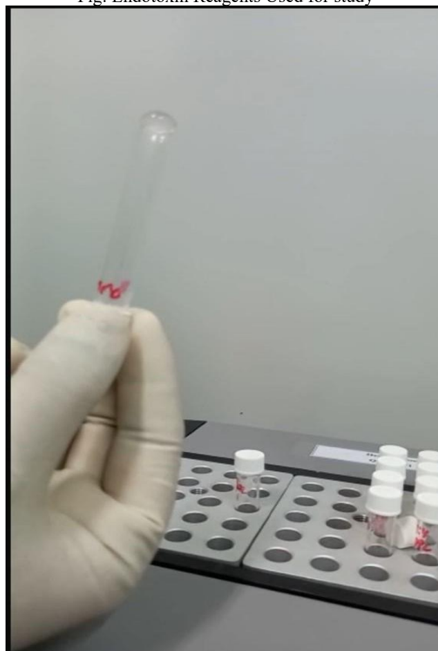
Fig: positive water control shows gel clot
